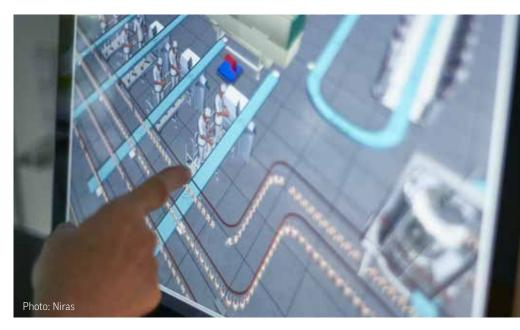
In one dairy assignment, a digital twin was used to validate and optimise the design of micro-dosing equipment for a new powder blending section. Bottlenecks were identified and removed, cutting the investment by EUR 630,000 in just three weeks of simulation work.
