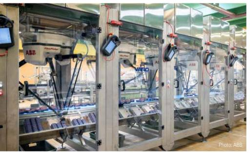
Up to 107 million cans of mackerel roll off the production lines at Sæby Fiske-Industri every year. A high-speed packing system, delivered by VARO, ensures each can is sorted and securely packaged before dispatch, primarily to supermarkets throughout Europe.
